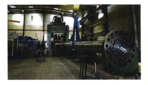
This was the case for the vessel »Commencement« that suffered an unfortunate grounding causing damage to the rudder system. For this job a new rudder stock Ø 336 x 7334 mm was manufactured as well as a new pintle and nuts. The rudder stock was delivered with 10 mm oversize, and MarineShaft service engineers were sent to location in Argentina to carry out conical boring of the rudder blade cones,
